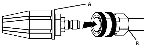
A - Turbo nozzle (boquilla turbo, buse turbo)
