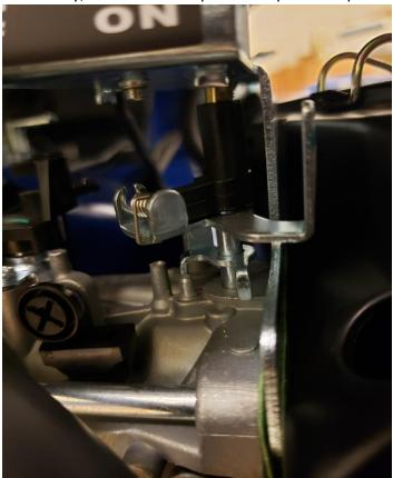
3. If everything is good to go on the motor, then unplug the 5-prong wire connector and test for power. First test the quick connect coming from the control module for power. This will determine if the control module is bad and not sending any power to the motor. If there is power coming from the quick connect then replace the stepper motor. Power readings should be around 7-10v on startup and 3v when running. Yellow and white are your power wires.
