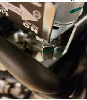
2. If the arm is free the next thing to check is the stepper motor. Make sure the shaft and spring are properly aliened. If neither are there or it seems like the motor is not seated all the way, then reline the parts or replace the parts.
