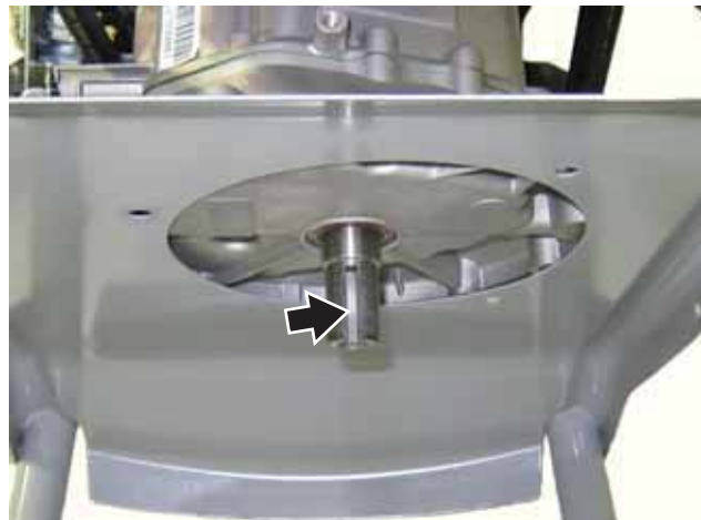
Figure 41 – Key and Crankshaft Keyway
