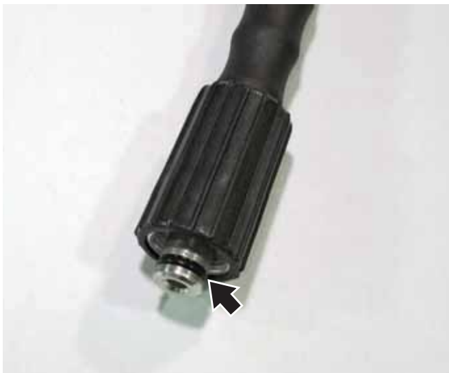
Figure 12 – High-Pressure Hose O-Rings
