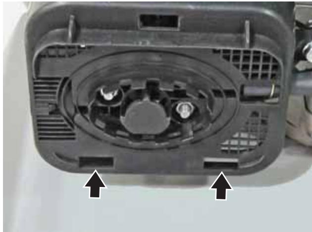
Figure 31 – Installation of Air Cleaner Cover
